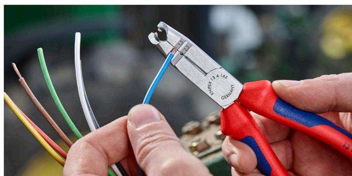
剥线孔用于1.5mm<sup>2</sup>和2.5mm<sup>2</sup>的导线
